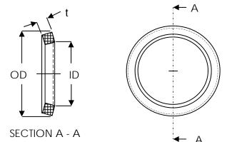
These preforms are designed specifically for SHP series feedthrus, ground pins and capacitors. They provide optimum flow and fillet when used with the recommended preform well and are available in three solders: Sn63, Sn96 and Sb5.
